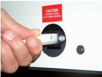
Connect the power cable to the SO100 so that you can open the door
