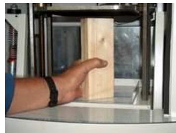
Before trying to start the machine, make sure the the wooden block has been removed from the machine itself
